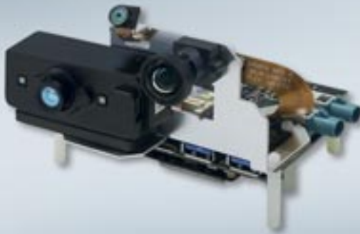
THUNDERCOMM's RB5 development kit with support for Sony's IMX577 camera module as well as the Omnivision OV9282 camera module which supports tracking applications, a TOF sensor accessory is also available from THUNDERCOMM.
