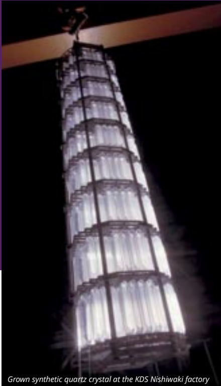
Grown synthetic quartz crystal at the KDS Nishiwaki factory
