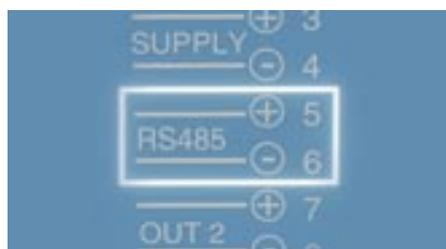
Modbus RTU is an open serial protocol derived from the Master/Slave architecture originally developed by Modicon (now Schneider Electric). It is a widely accepted serial level protocol due to its ease of use and reliability. Modbus RTU is widely used within Building Management Systems (BMS) and Industrial Automation Systems (IAS).
