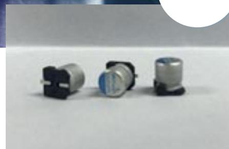
SUN Electronic Industries Corp. (SUNCON) has added small dimension versions with a diameter of 5mm only to their 125°C/4,000hrs-series HVPF and HVPC. Thus, the advantages and features of electrolytic-hybrid capacitors can also be used in a smaller space.
