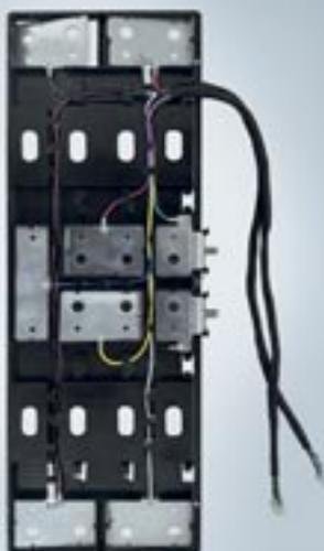
Figure 3: Cells Contact System
