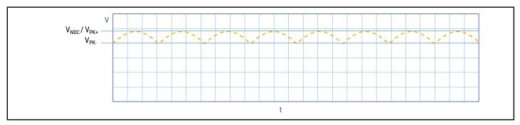
The applied peak-to-peak ripple voltage shall not exceed 0.2 x  $V_{\text{NDC}}$ . The peak voltage shall not exceed the rated voltage  $V_{\text{NDC}}$ .
