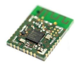
The OSB-DA14585 RF module are designed in compliance with the Bluetooth 5.0 LE Specification and is based on the Dialog DA14585 single-chip controller. The new Bluetooth 5.0 features enable a higher symbol rate of 2 Mbps and open field transmission rage up to 90 meters.
