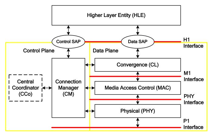
Figure 1 HPAV Architecture
