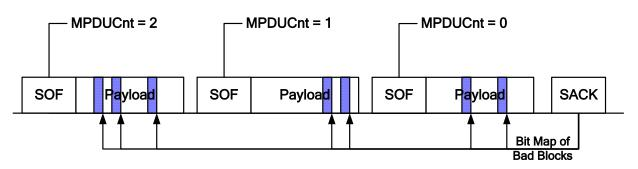
Figure 4 MAC Segmentation and MPDU Generation
