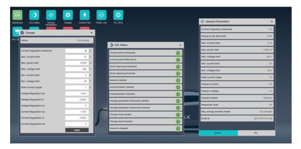
Furthermore the user gets full control about the simulated charging process. All relevant parameters can be configured via the Web Application. An integrated PID-controller controls current and voltage of the simulated charging process and its parameters can also been configured via the Web Application (EVSE version).
