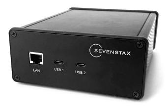
remote station. The V2G simulator further conforms to the norms by supporting Powerline Communication (HPGP including SLAC) and IEC 61851 Control Pilot (CP) handling (pulse width modulation, voltage reading/control).
