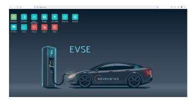
User guidance takes place via a convenient Web Application on your browser. During operation, the PLC communication can be mirrored to an Ethernet interface and analyzed using SEVENSTAX GreenShark (optionally available). It is furthermore possible to integrate the V2G simulator into an automated test system via the HTTP/JSON interface.
