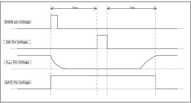
Fig.8 Operation after shutdown
