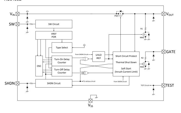
\*Diodes inside the circuit are an ESD protection diodes and a parasitic diodes.
