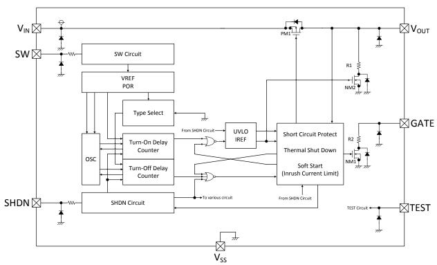
Fig.1 XC6193A Block diagram
