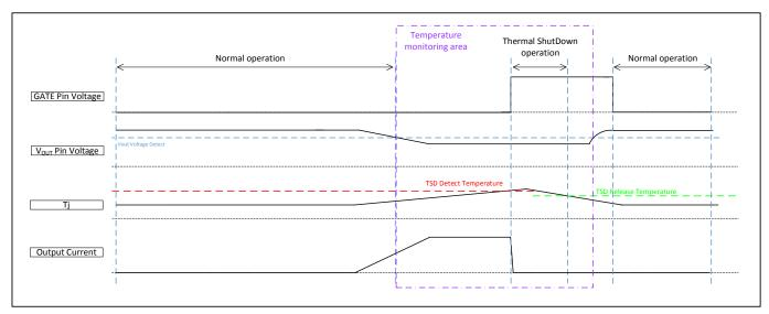
Fig.9 Thermal shutdown function
