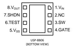
\*The dissipation pad for the USP-8B06 package should be solder-plated in recommended mount pattern and metal masking so as to enhance mounting strength and heat release.
