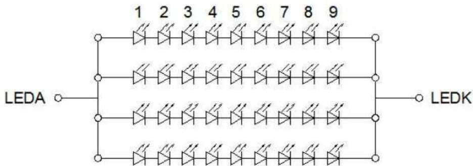
Fig. 3-1 LED test circuit diagram
